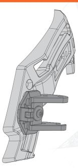
5 Reinstall center screw. Torque to 16-18 in-lb. When properly tightened, AMP™ Helmet Adapter Arm assembly will not slide on rail. It should only be able to pivot. DO NOT OVER TIGHTEN.
